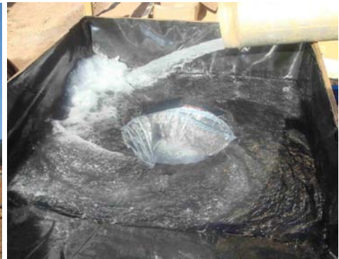
Area Inlet Simulated Showing Influent Discharge From Pipe
