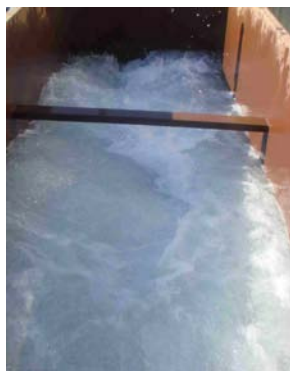
Inside View of Hopper Agitator
