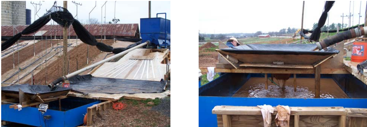
Figure 1. Test set-up, including mixing tank and wooden box with simulated area inlet inside collection tank. (typical grab sampling shown)
